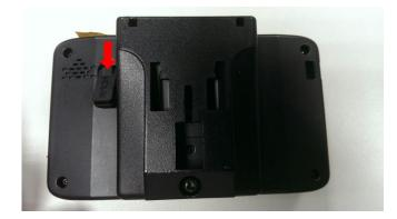
Then push down the bottom of rubber cover to close it.
