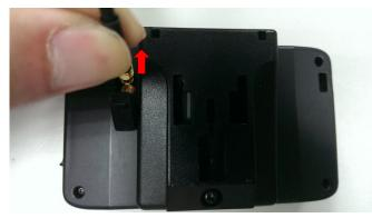
4. Push down the top of rubber cover into antenna jack first.
