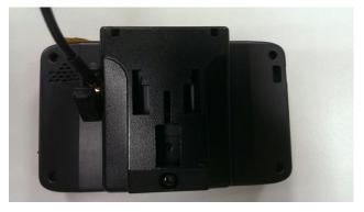
3. When unplugging the external antenna, hold the connector and unplug it vertically.
